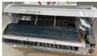
3. Remove the cover by removing these 10 screws.
