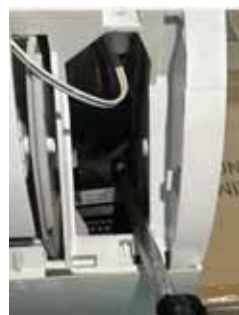
3. Remove leak sensor.
