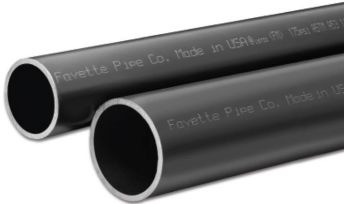
Produced to the latest revision of ASTM A53A/53M - ASME B36.10M. Sch 40 is available in 1/2" to 2" dia. and in 10' and 21' lengths in PE, T&C, TBE, and grooved ends.
