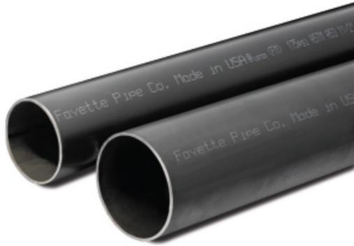
Suitable for welding or roll grooving, ASTM A795/A135. Sch 7 is available in 21' lengths, diameters of 1-1/4", 1-1/2", 2", and 2-1/2".
