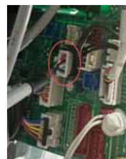
4. Pull out the PCB and unplug the refrigerant leak sensor from CN3.
