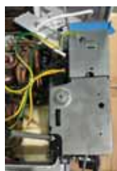
4. Remove the electrical box cover.
