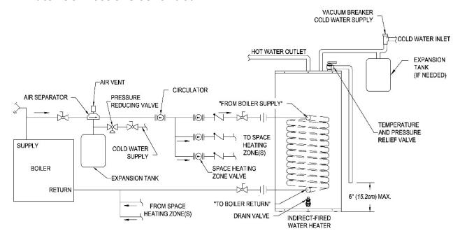
Figure 4 - Water Boiler Piping with Circulators
