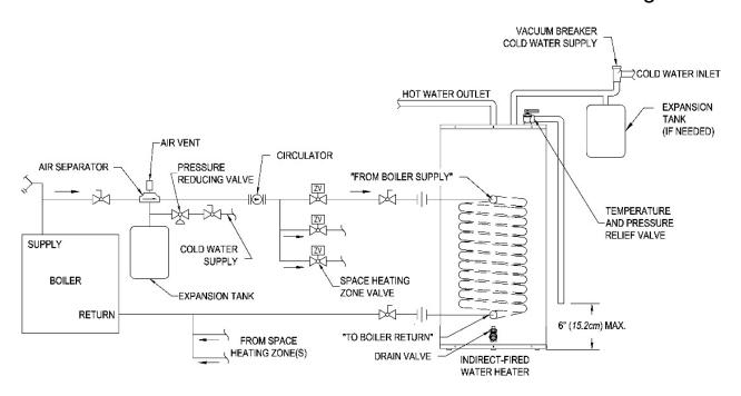
Figure 3 - Water Boiler Piping with Zone Valves
